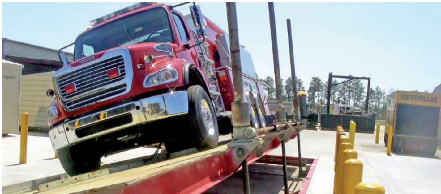
The tilt table is moved to 26.5 degrees in both directions
